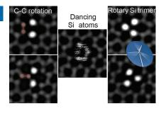
Atomic competition: The dynamic atomic processes during the formation of a rotary Si trimer in monolayer graphene were monitored using aberration-corrected scanning-transmission electron microscopy. An incoming Si atom competes with and replaces a metastable C dimer next to a pair of Si substitutional atoms at a topological defect in graphene, producing a Si trimer.
