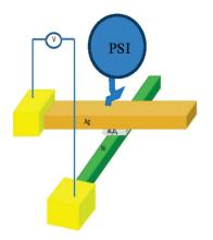
Unexpected influence: By using a newly developed spintronic device it is shown that the electron transfer (ET) efficiency of photosystem I (PSI) is affected by the electrons' spin. High-spin selectivity is found throughout the entire ET path, and the spins of the electrons being transferred are aligned parallel to their momenta.
